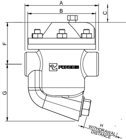
Figure 2 : Dimensional Drawing of FMBT50
