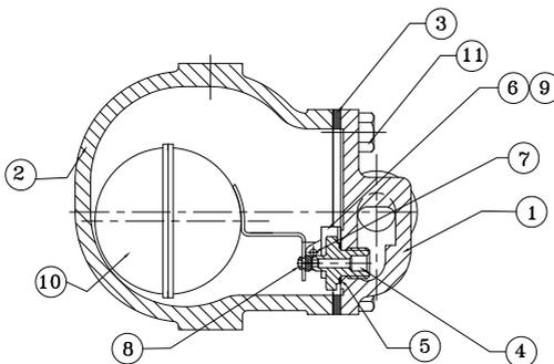
Figure : 1: Single Orifice Float Trap With SLR
