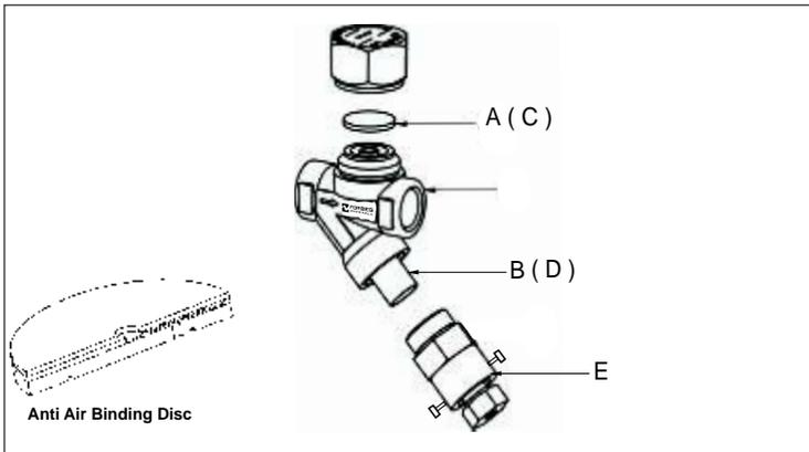
Figure 5: Parts Available as spares (Heavy outline) for FMTD65-B
