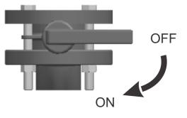
Check that the isolation valve on the pump is in open condition and observe the pump performance.
