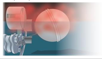
When the condensate load is higher, additional lift of the float causes the second orifice to open, thereby enabling the TOFT / CMTOFT to handle both start up and running conditions effectively.
