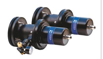
Provides non-contact measurement of flue gas velocity using a time-delay correlation of the flue gas infrared energy sensed by two detectors spaced at a known distance apart
