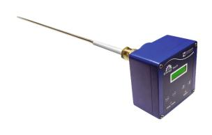
EnergyTech 301 dust monitor uses the well proven tribo electric sensor technology to directly measure particulate concentration by sensing the frictional charge created when particles collide with conductor, i.e metal probe.
