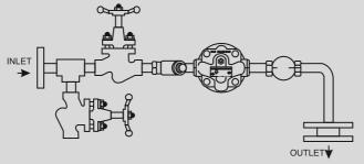
Single Orifice Float trap module
