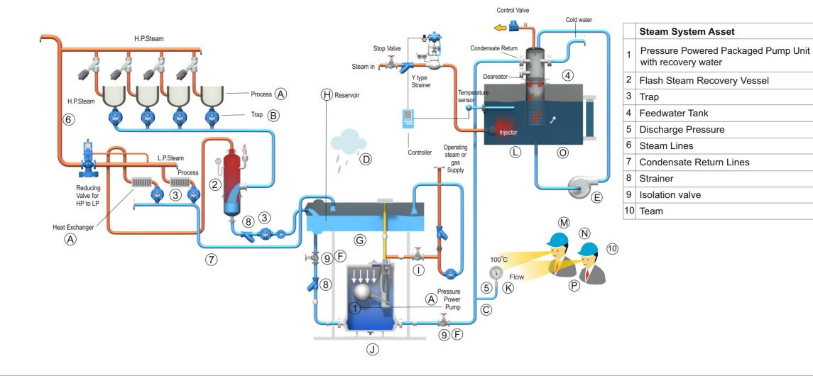
The condensate system relies on traps and pumps to get condensate back to the feedwater tank where it can save the most energy and water stress.
