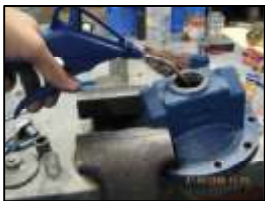
Blow debris from body & reassemble.
