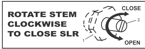
Figure 7: SLR setting for only SLR and SLR+TV configuration
