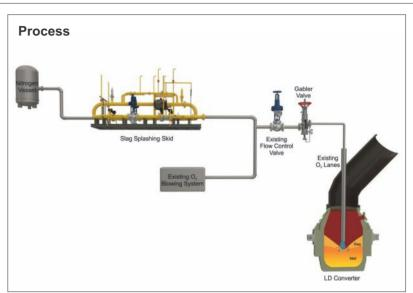
Slag splashing is a powerful technique available to steelmakers for increasing the lining life of LD converters, maximising production from the existing equipment and reducing refractory and gunning cost.
