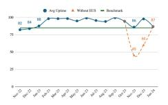
In October 2023, the probe experienced unnecessary choking, causing uptime to drop from 89% to 86%. Due to the plant being digitally enabled, real-time digital monitoring helped the issue to be immediately identified and corrected. Without this digital intervention, the problem would have remained unnoticed, potentially dragating uptime down to as low as 45%.
