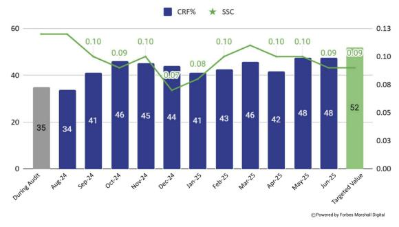
Reducing specific steam consumption and improving condensate recovery factor using EverSense for Plant-wide Performance, a Forbes Marshall Digital solution
