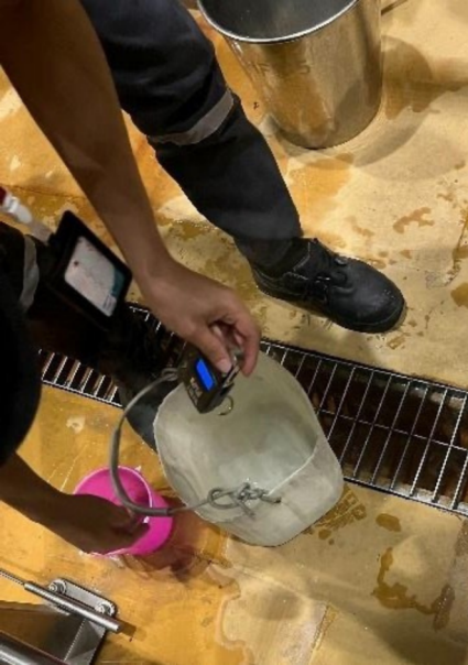
Condensate trials at the Pasteuriser Hot Fill line 3 with the plant team
