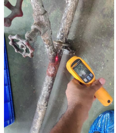
125°C (257°F) observed temperature in common condensate line
